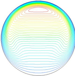
**FIGURE 2.** Typical isotherms at low Rayleigh numbers
