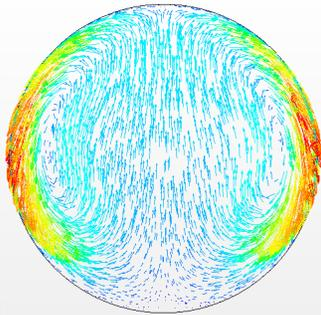
**FIGURE 3.** Typical velocity distribution at low Rayleigh numbers
