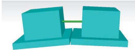
Figure 2: Two adjacent structures with commodities running between them with tilt.
