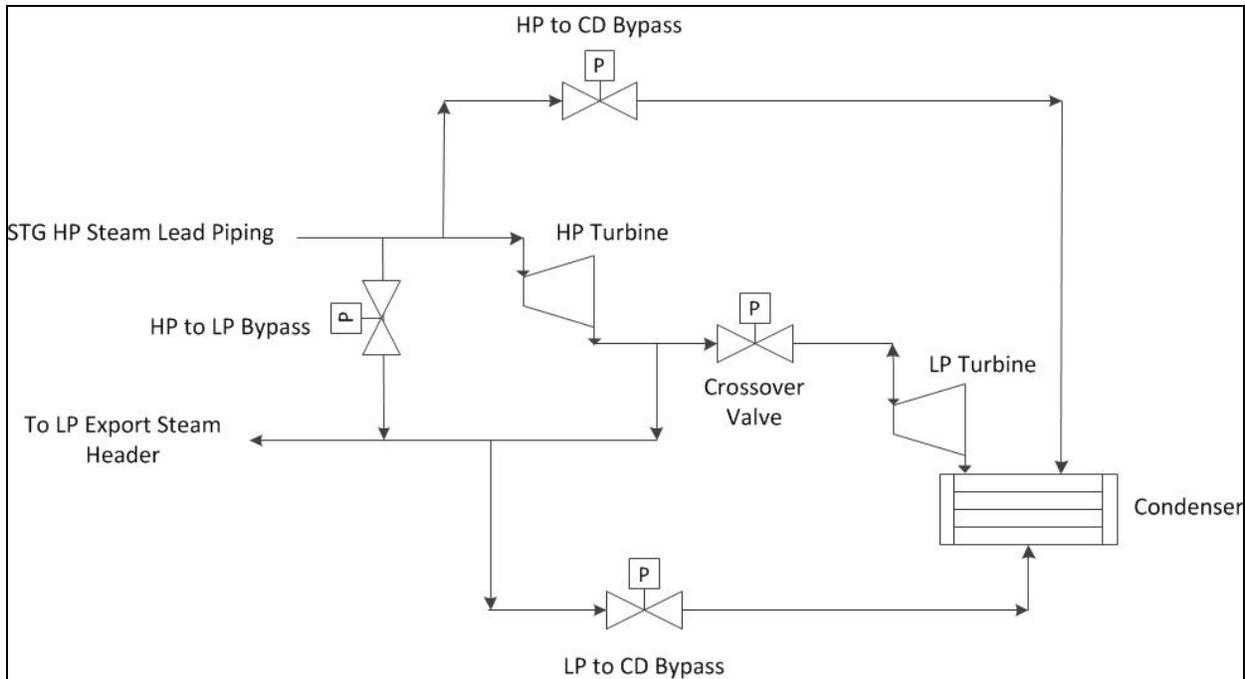
**Figure 3 STG HP and LP Piping Schematic**
