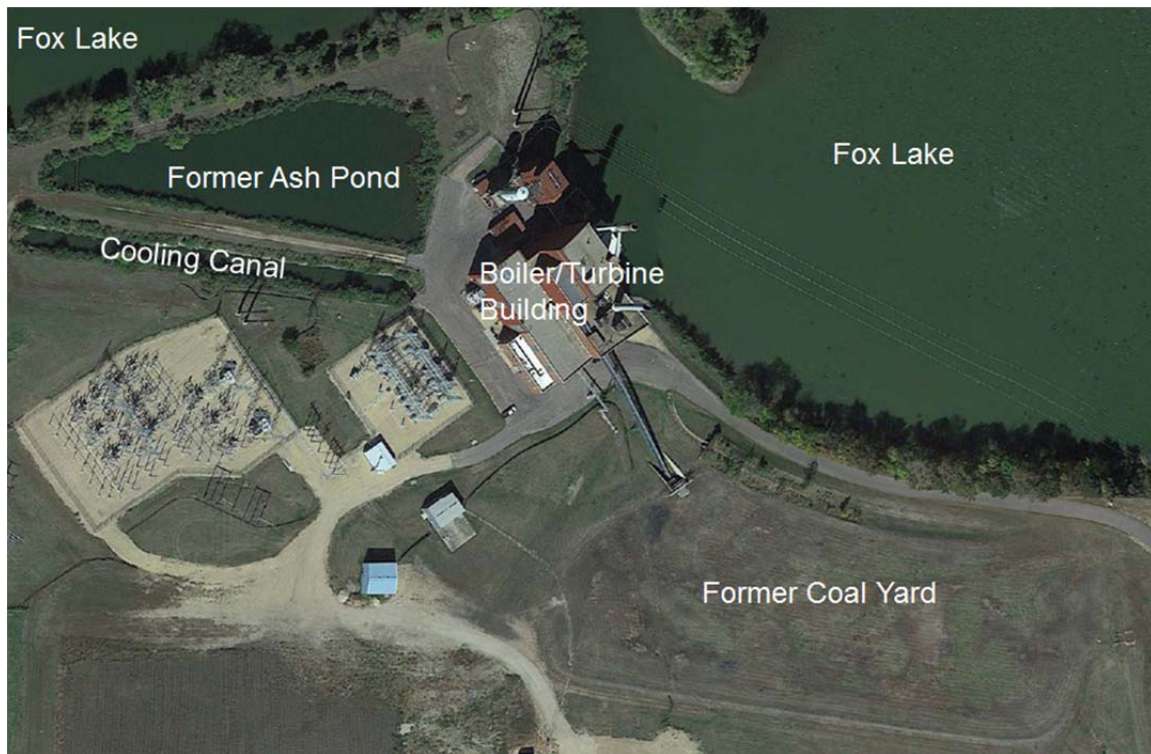
Figure 1: Annotated aerial photograph of the Fox Lake Generating Station prior to Clean Closure Project.
