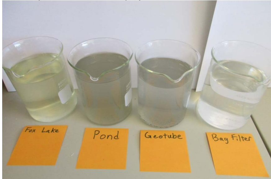
Figure 4: Water clarity at various locations throughout the dredging and filtering process.
