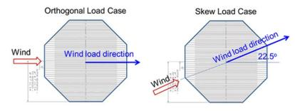
For octagonal wind turbine foundation footings with orthogonally oriented reinforcement, we have performed parametric studies that consider a skewed wind-load case to evaluate the flexural capacity of an octagon spread footing foundation's top and bottom steel reinforcement.
